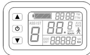
The metric units will be set after finishing setting wheel diameter, Km/H and Km or MPH and Mil flash. Hold ▲ or ▼ shortly and select the metric units of speed and mileage in synchronization.
