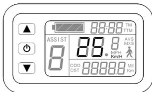
After power on for 5 seconds, hold ▲ and ▼ at the same time, maximum riding speed Km/H flash, hold ▲ or ▼ shortly to set the maximum riding speed (default 25Km/H). Hold ⏻ button shortly and go to the next parameter settings.
