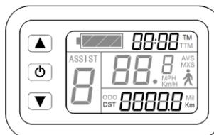
After power on for 5 seconds, hold and at the same time, single trip riding time (TM) and single trip distance (DST) flash, hold button shortly, the content of both is cleared. If failed holding the button within 5 seconds, it will automatically return the display interface after 5 seconds, original content is preserved.
