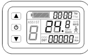
In the display of total trip time and distance, hold or shortly to display of single maximum speed (MXS) and average speed (AVS). hold button shortly again to return the display interface. In the riding condition, 5 seconds later,
