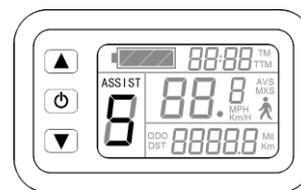
Hold or shortly to switch 1-5 file gear. Gear 1 is for the minimum power, gear 5 is for the highest power. Each startup will automatically restore the gear shutdown last time. Gear 0 is without booster function.
