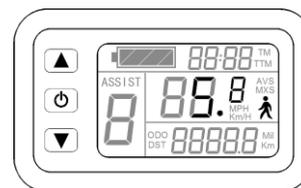
Hold and flashes, the vehicle drives at the speed not more than 6Km/h. Release button, the function is invalid.
