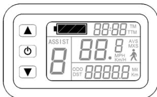
The meter can automatically identify the battery capacity when the battery capacity indicator is supporting use with the specified controller. When the battery capacity is over 70%, the four power displays of the meter are lit, and the battery capacities drop, the four power displays are off in order, when
